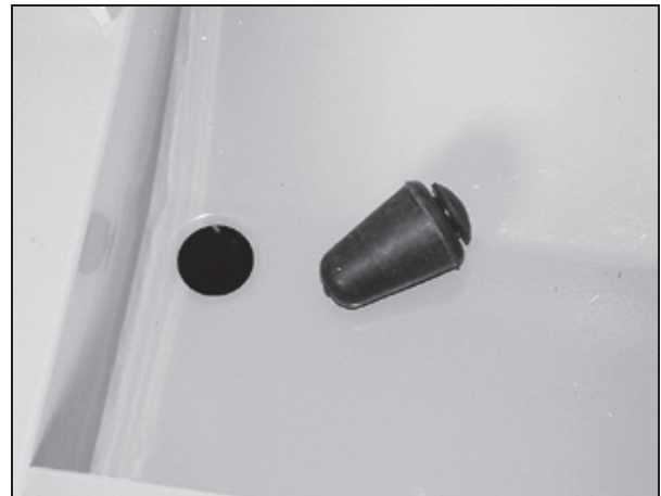
Fig. 3.9 Drain hole in the water trough (with plug)
