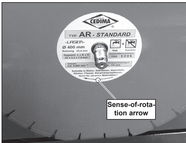
Fig. 3.12 Sense-of-rotation arrow on the blade
