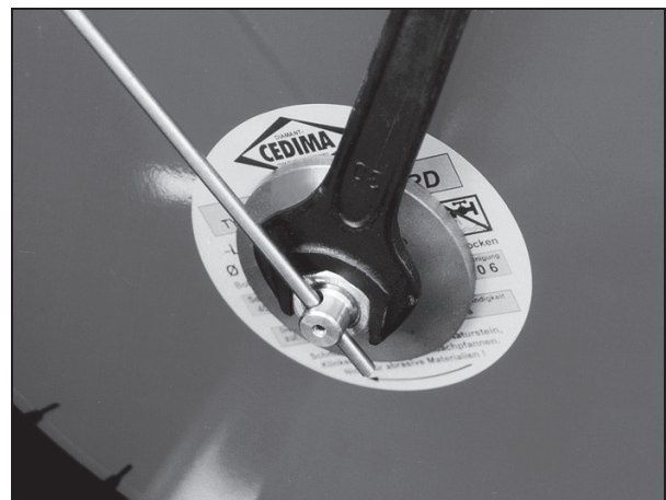
Fig. 3.15 Locking the saw blade using the mandrel and spanner
