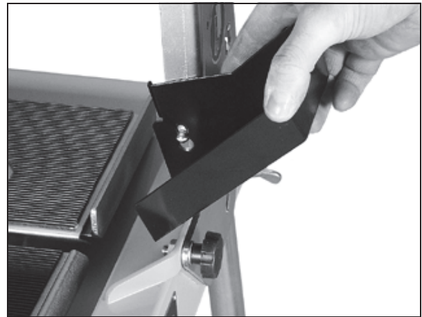
Fig. 3.2 Installing the front splash guard
