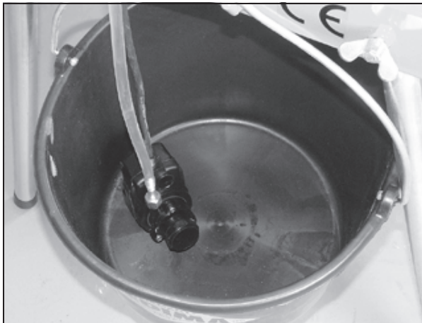
Fig. 3.8 Wet-pit- (water-) pump in the bucket hanging below the frame
